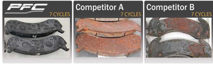
*GM9540P Accelerated Corrosion testing cycles
